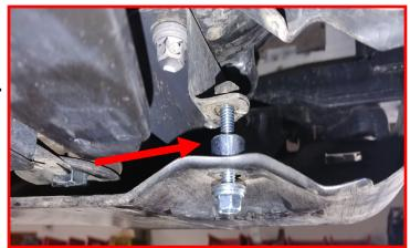
Move to the suspension, remove the sway bar end link from the knuckle. Let hang out of the way.
