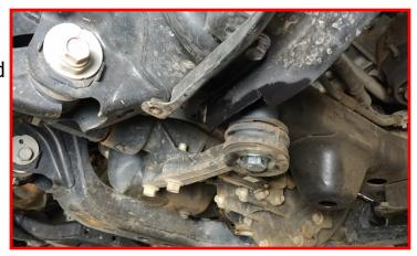
If equipped, install the differential gravel guard to the rear most cross member with the factory hardware and the front cross member with the provided hardware and spacers. Torque to 5 ft-lbs. (Driver side shown)
