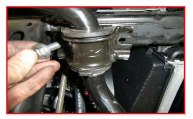
Install the ReadyLIFT sway bar brackets to the frame using the factory hardware. Torque to 35 ft-lbs.
