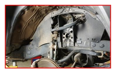
Install the ReadyLIFT strut extension to the strut using the factory hardware. Torque to 30 ft-lbs.
