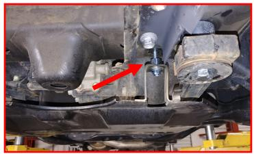
Install the front gravel guard to the core support cross member using the factory hardware. Do not tighten at this time.
