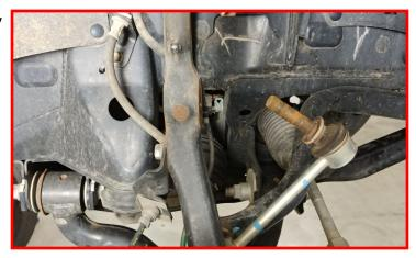
Remove the lower strut hardware.
