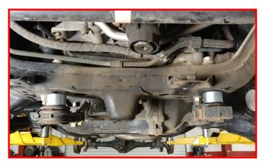
Install to the frame using the provided hardware and the factory large bushing washers in their original location. Torque to 95 ft-lbs.
