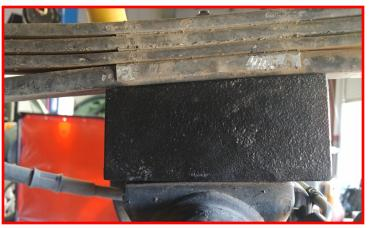
Install the shock lower hardware. Do not tighten at this time. Install the wheels and lower the vehicle to the ground. Jounce the vehicle to settle the suspension to the new ride height. Torque the lower shock hardware to 45 ft-lbs, and the u-bolts to 110 ft-lbs.
