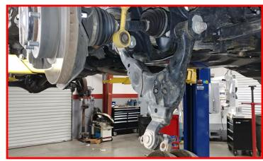
Remove the strut from the vehicle.
