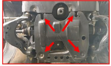
Locate the front gravel guard mounts on the frame. Look to see if there will be any clearance issues with the front differential mount when it is lowered. (Driver side shown.)
