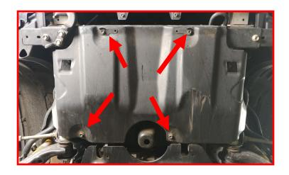
If equipped, remove the differential gravel guard.
